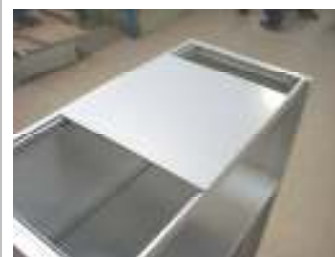
Fit the fitted shelf blocks underneath the lip of the rear of frame, and lower shelf onto the front of the frame.
