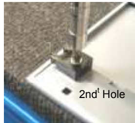
Fit both plastic guide blocks on one side of shelf as above.
