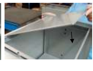
Fit the fitted shelf blocks underneath the lip of the rear of frame, and lower shelf onto the front of the frame.
